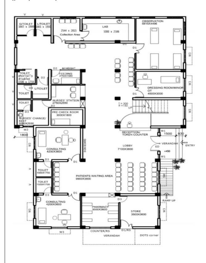
GROUND FLOOR PLAN SCALE 1:100 ALL DIMENSIONS IN MMS
